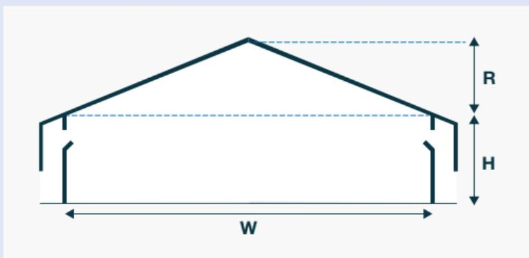
**Cross section area =  $0.5 \times W \times R + W \times H$ .**
