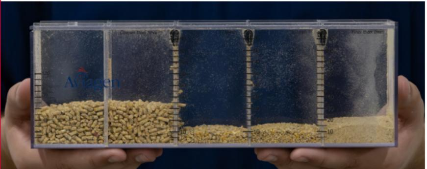
**Recommended particle size distribution for crumble or pelleted feeds.**
