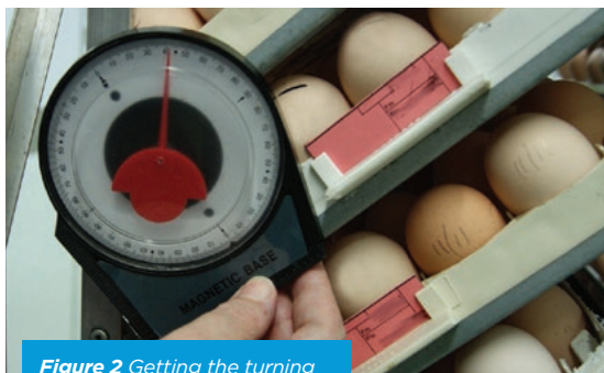
Figure 2 Getting the turning angle just right at 42 degrees.
