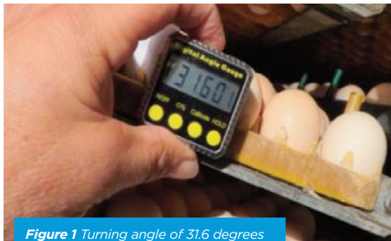
Figure 1 Turning angle of 31.6 degrees is too shallow. Target is 40-45 degrees.
