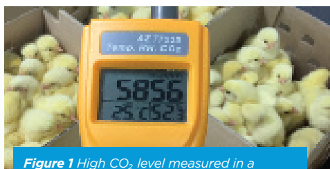
Figure 1 High CO 2 level measured in a holding room with insufficient ventilation.
