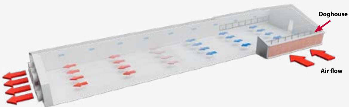
Figure 6.18 Air flow in a tunnel-ventilated house.
